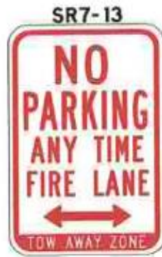
FIGURE 503.3 FIRE LANE SIGNS
